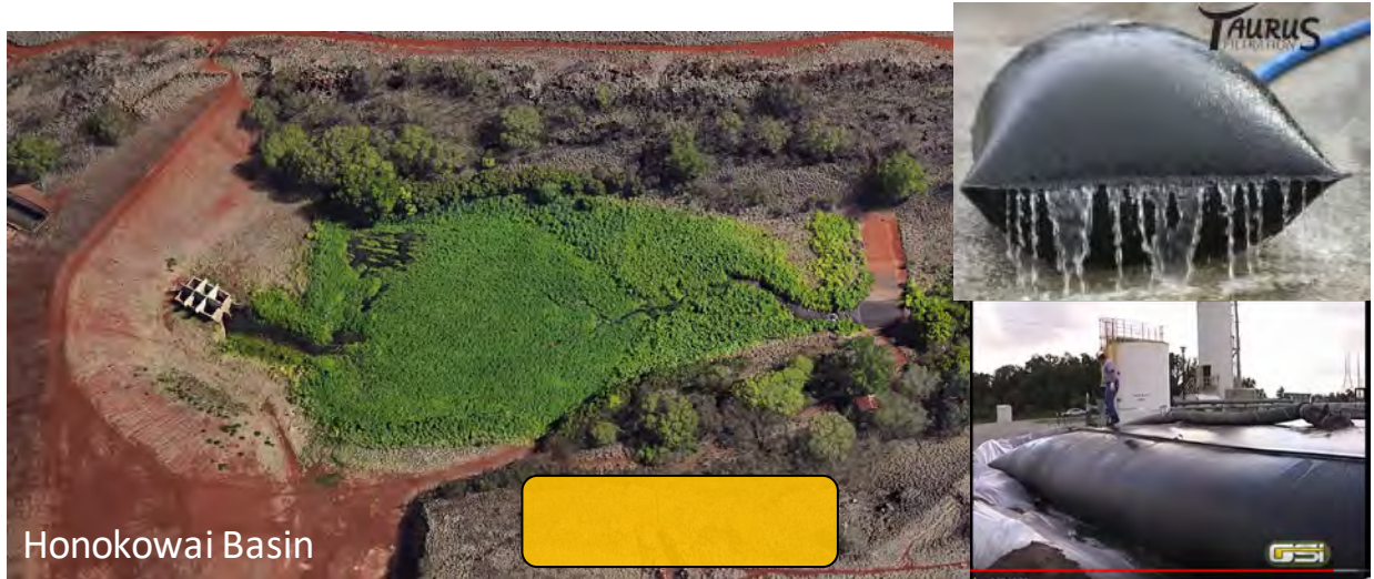
Figure 3- 15 Geotextile Filtration. USACE concept illustration. Example of current application to the right. Potential location (yellow polygon).
